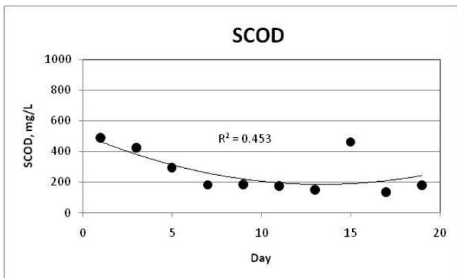
Fig. 2 Reactor effluent soluble chemical oxygen demand SCOD of master culture semi continuous batch anaerobic acetogenic reactor.
