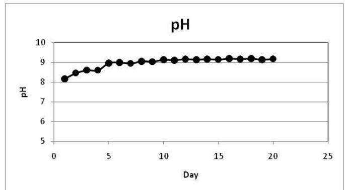
Fig. 4 Reactor effluent pH of master culture semi-continuous batch anaerobic acetogenic reactor.
