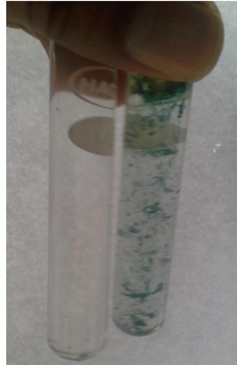
Fig. 5 Picture of raw wastewater against treated effluent clearly showing visually the success of the treatment process.
