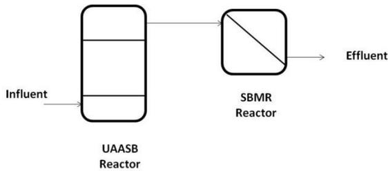
Fig. 1 Schematic flow diagram of the proposed, modified treatment train for wastewater treatment from textile processing facilities. UAASB stands for up-flow anaerobic acetogenic sludge blanket reactor and SBMR stands for sequential batch membrane reactor.
