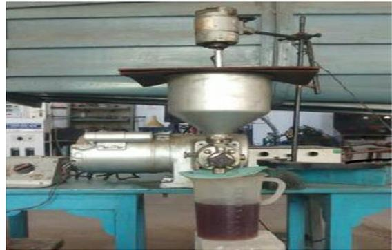
Fig. 3. Blending Machine Apparatus
