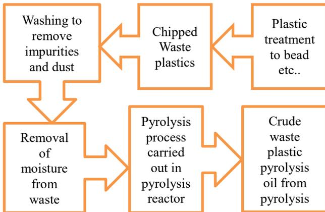
Fig. 1. Waste plastic pyrolysis process
