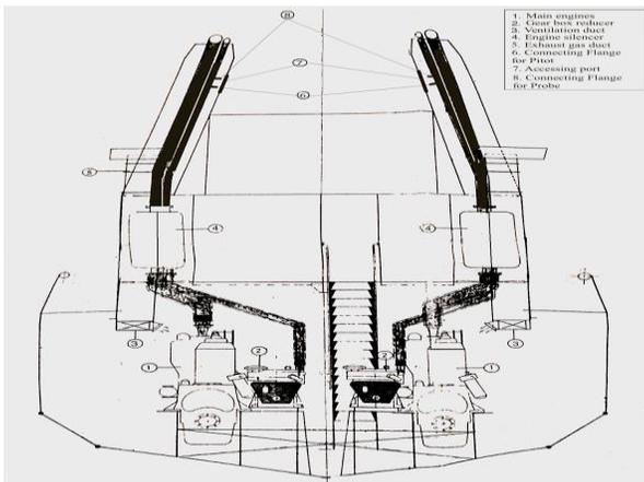
Fig. 5 Sectional Elevation of the experimental vessel [15]
