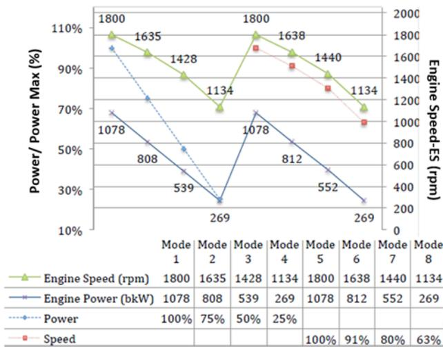
Fig. 6 Engine Performance for different Operating Modes
