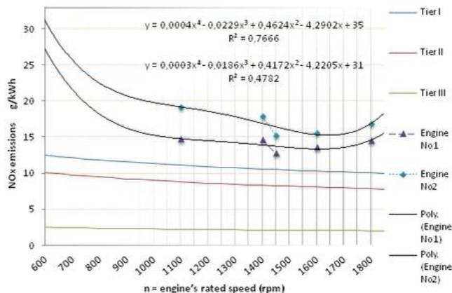
Fig. 9 The NOx production behavior after using the adBlue liquid
