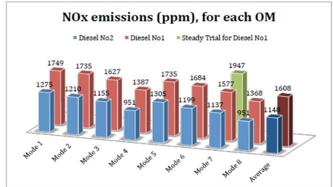
Fig. 7 NOx Emission levels produced by the two diesel engines under different operating modes
