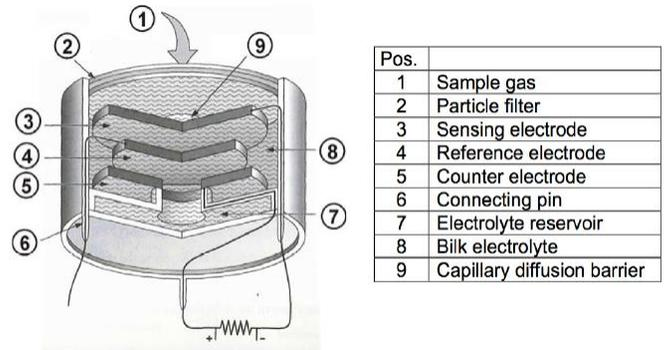
Fig. 3 Electrochemical sensor of the VarioPlus [12]
