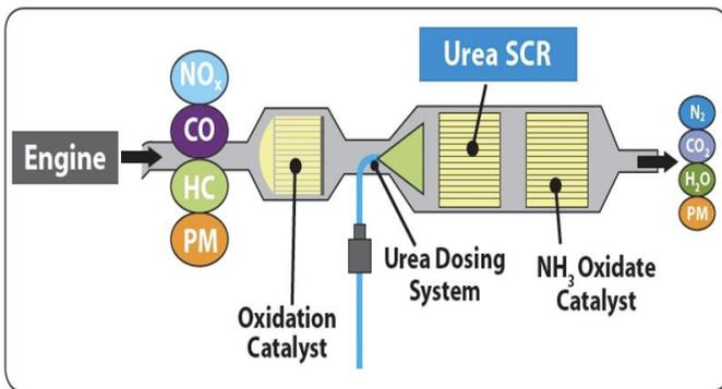
Fig. 2 Typical Selective Catalytic Reduction set up [10]
