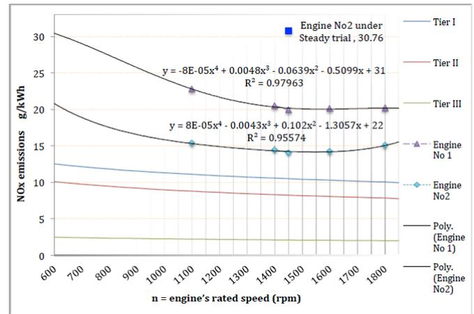
Fig. 8 Engines NOx specific emissions (g/kWh) in comparison to Tier I, II, III
