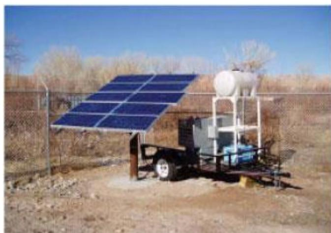
Fig 3. Mobile solar powered reverse osmosis
