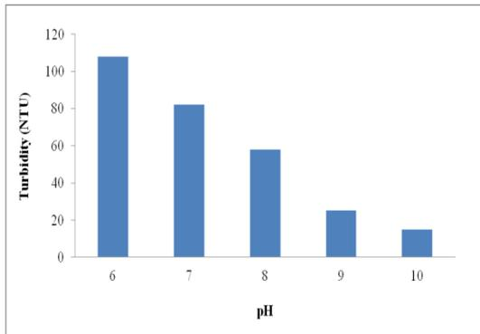
Fig. 3 Residual turbidity of treated wastewater at different medium pHs
