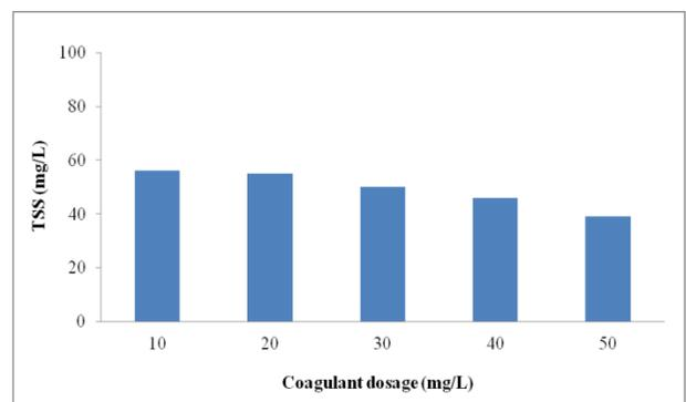
Fig. 2 Residual TSS of treated wastewater at different coagulant dosage
