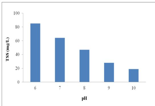
Fig. 4 Residual TSS of treated wastewater at different medium pHs
