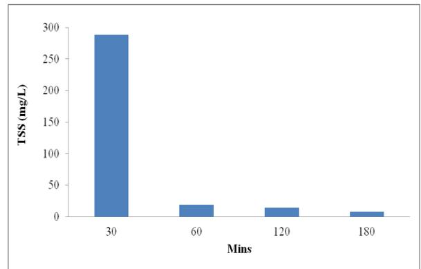
Fig. 6 Residual TSS of treated wastewater at different settling time period
