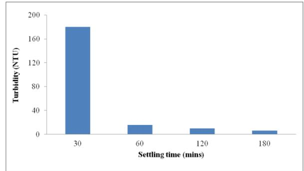
Fig. 5 Residual turbidity of treated wastewater at different settling time period
