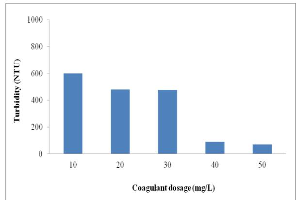
Fig. 1 Residual turbidity of treated wastewater at different coagulant dosage
