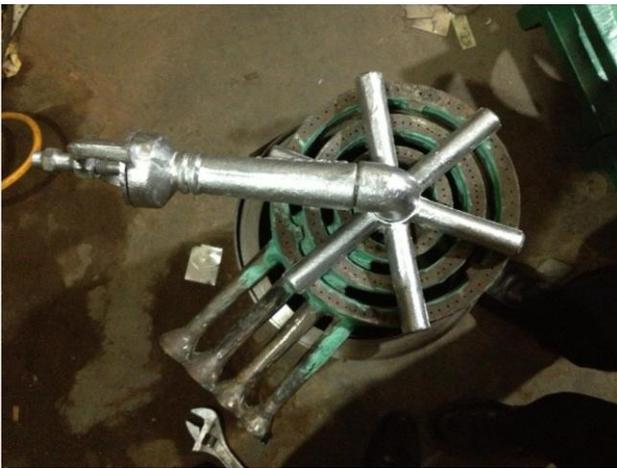
Figure 3. The purpose designed energy efficient burner developed in this study with the Star burner superimposed on it showing the effective area increase in direct flame coverage.
