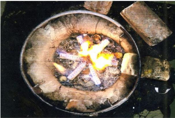
Figure 1. The existing Star Burner in use showing the inefficient operation due to inherent design flaws leading to low thermal efficiency and high consumption of fuel.
