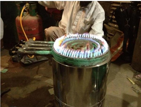
Figure 2. The purpose designed energy efficient burner developed in this study showing clean burning with effective coverage with optimum flame throwing angle leading to high thermal efficiency and low consumption of fuel.
