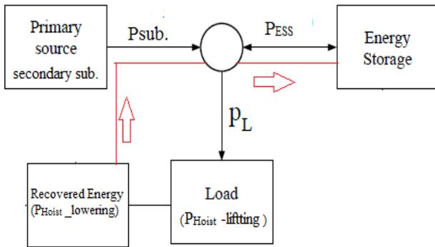
Fig. 4: Topology of the power system (First model).
