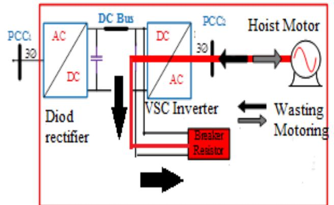
Fig. 3: Simplified Diagram of the main components of eRTG crane.
