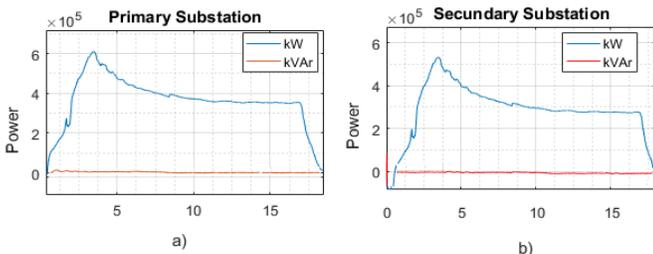
Fig. 9: The primary and secondary substation peak performance with an AFE and ESS (First Model).
