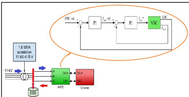
Fig. 5. Voltage source converter control system used in the model [6].
