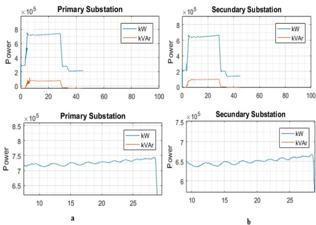
Fig. 8: The primary and secondary substation peak performance without an AFE and ESS.
