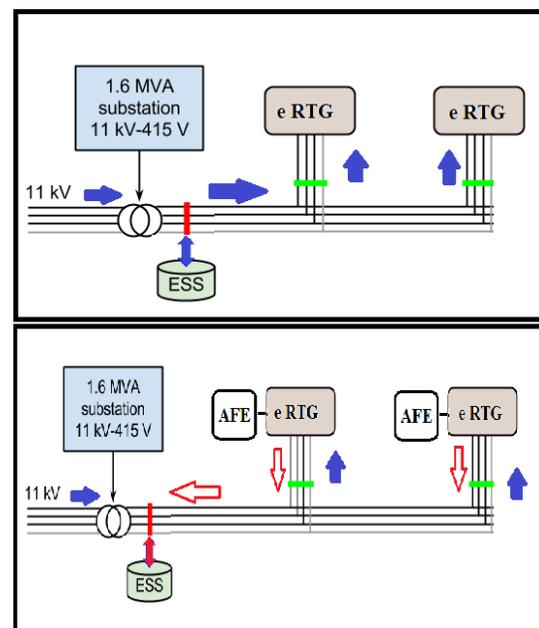
Fig. 1. Diagrams of two Cranes equipped with / without AFE and ESS.
