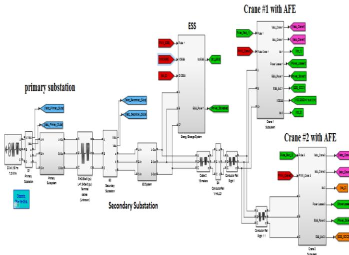
Fig. 7: Simulink model of network of cranes equipped with an AFE and ESS (First model).
