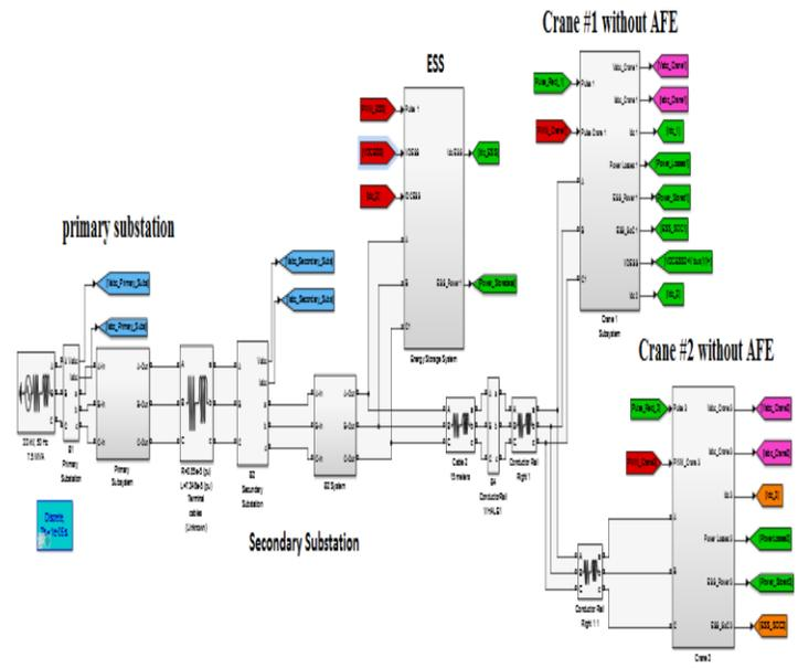
Fig. 10: Simulink model of network of cranes equipped with ESS and without AFE (Second model).
