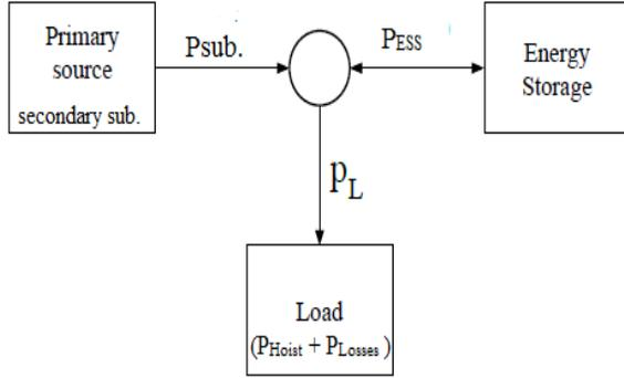
Fig. 6: Topology of the power system (Second model).
