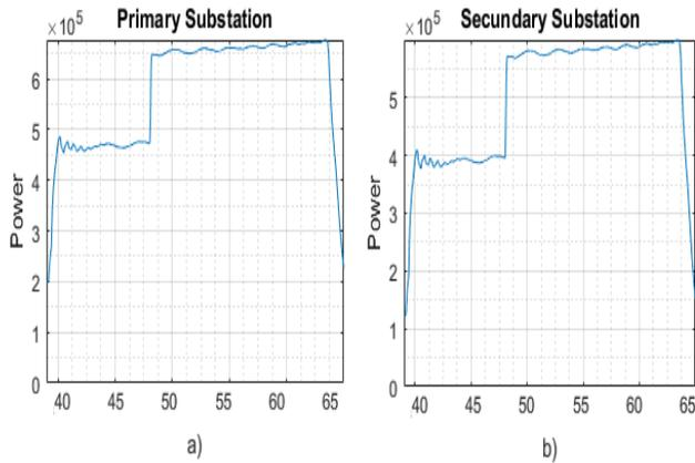
Fig. 11: The primary and secondary substation peak performance with ESS and without an AFE (Second Model).
