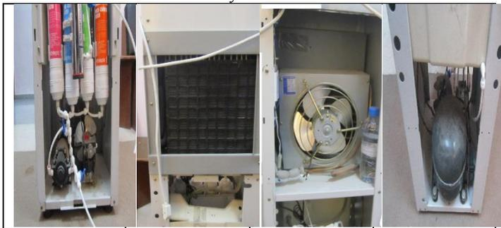
Fig. 2 Air water-generating components (electrostatic filter, UF Cartridge Filter, fan, condensation unit, and compressor).
