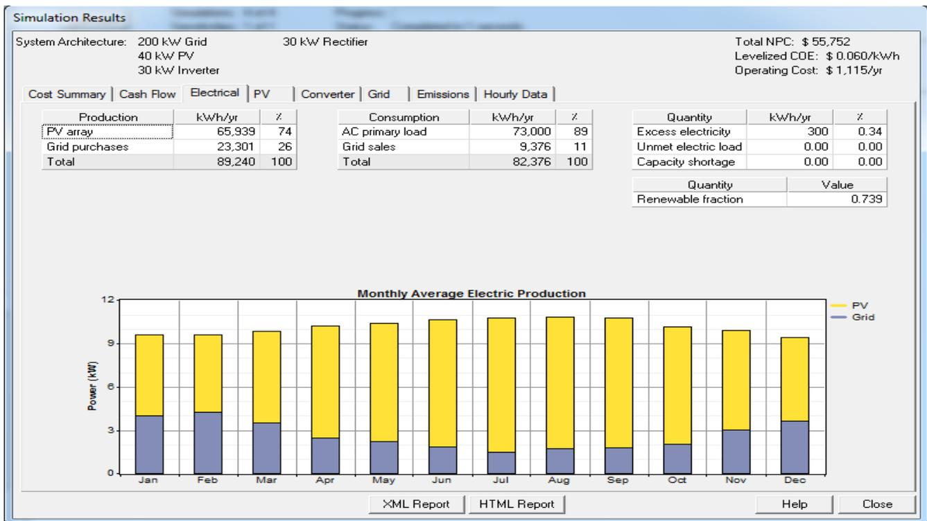
Fig. 5 40 KW Photovoltaic (PV) simulation result.
