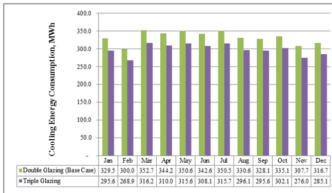
Fig. 5 Monthly cooling energy consumption (MWh) of models with base case and proposed glazing configurations
