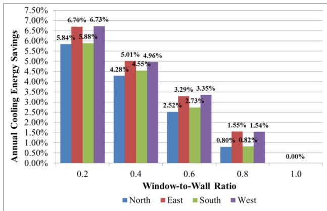
Fig. 4 Annual cooling energy savings by different WWR at different façade orientations
