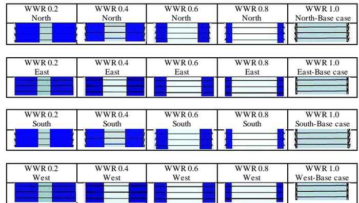
Fig. 3 Proposed WWR at different façade orientation
