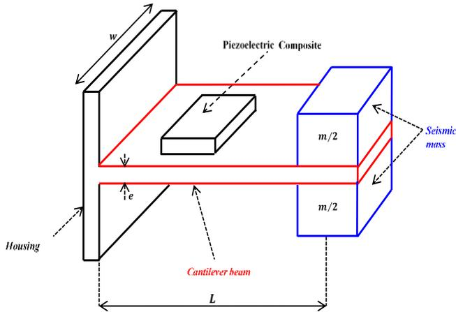
Fig. 4 Geometry of the cantilever piezoelectric transducer
