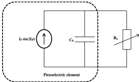
Fig. 7 Piezoelectric element model with resistive load
