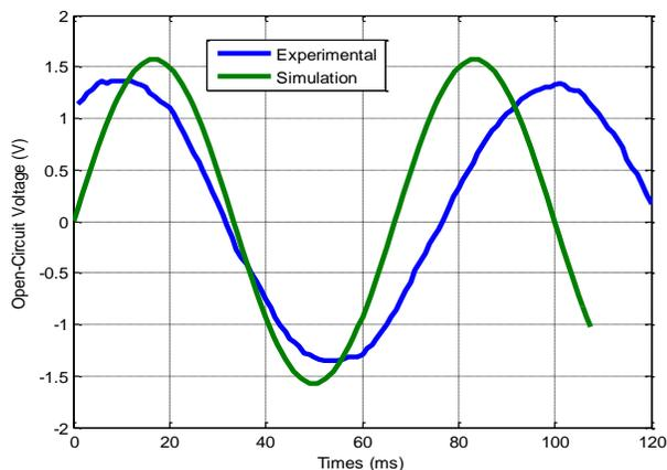
Fig. 10 Experimental and simulation waveform of Open-Circuit Voltage
