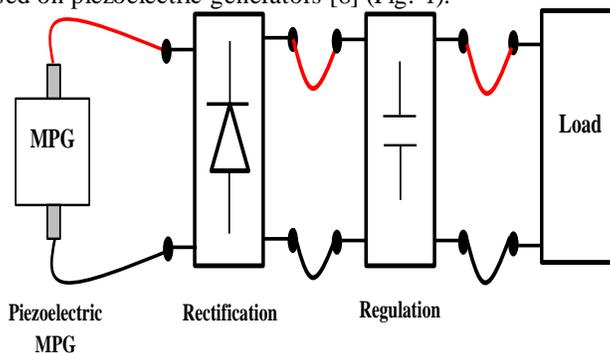
Fig. 1 Piezoelectric harvesting general architecture
