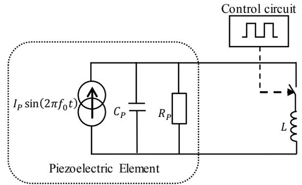
Fig. 1 Piezoelectric transducer with SSHI technique
