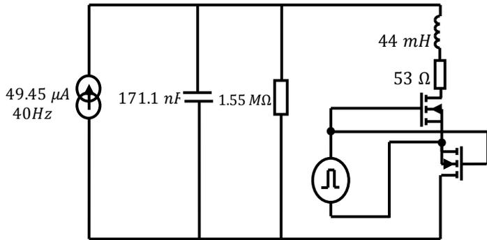
Fig. 6 Transducer model and SSHI stage
