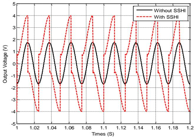
Fig. 7 Open circuit voltage of transducer
