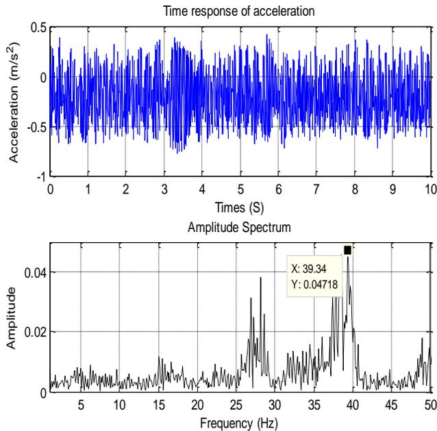
Fig. 3. Detected vibration at 2000 tr/min engine
