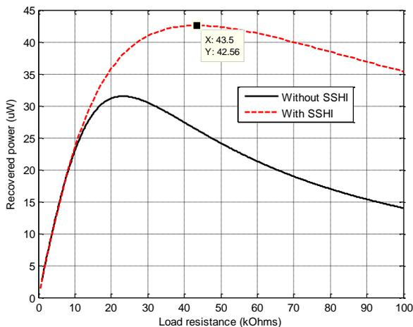
Fig. 8 Variation of power as a function of load
