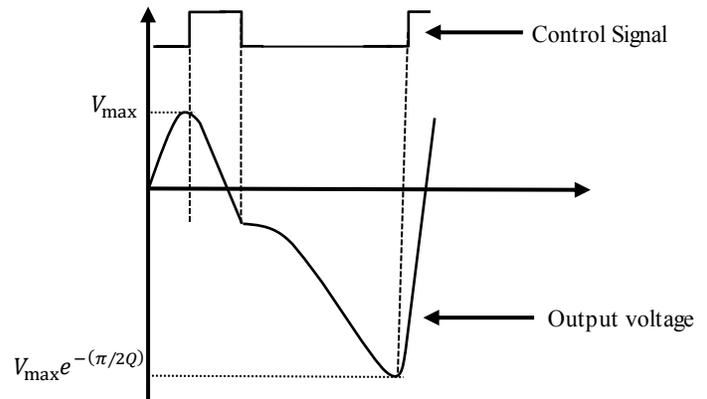
Fig. 2 SSHI waveforms
