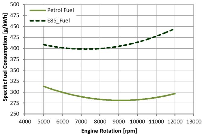
Confirming the simulation results, the increase in the specific fuel consumption relays between 30 and 45% for the tested range (5000rpm to 12000rpm), presenting higher differences for higher regimes.
