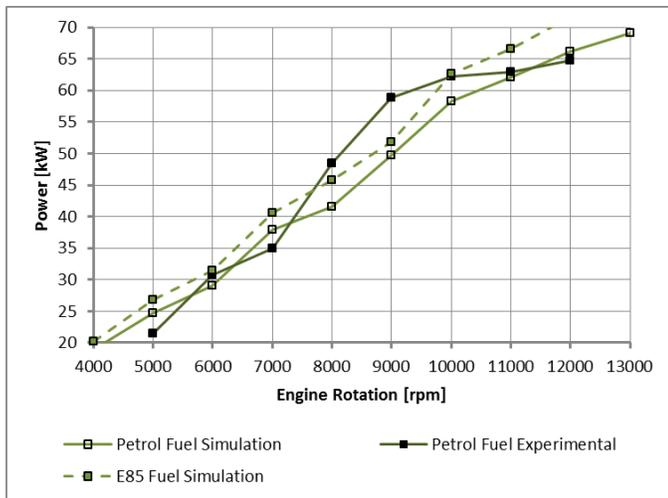
Figure 3 – Comparison engine power curves with petrol fuel obtained in simulation software and experimental tests.
