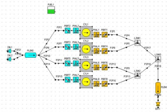
Figure 1 – Suzuki's engine model created in LES.
