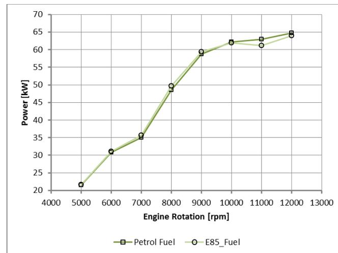
Figure 5 – Comparison engine power curves with petrol fuel and E85 obtained in experimental tests.
