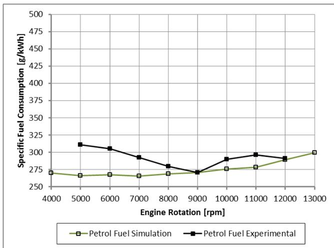
Figure 4 - Comparison between specific fuel consumption with petrol fuel obtained in simulation software and experimental tests.
