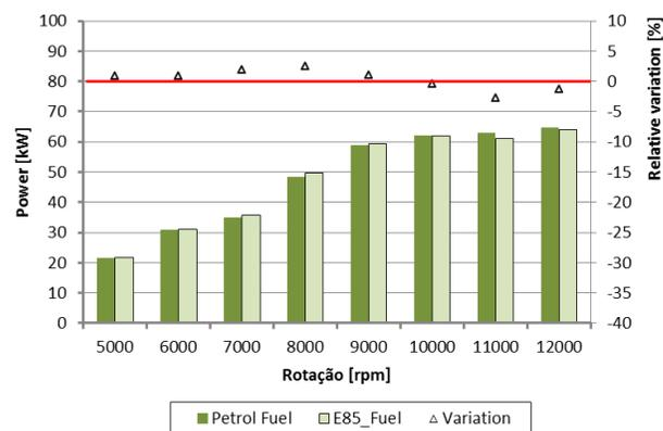
Figure 6 – Variations between engine power results considering petrol fuel and E85 in experimental tests.
