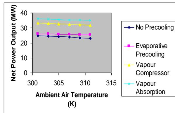
Figure 7: Comparison of Net Power Output for various precooling techniques at different ambient air temperatures
