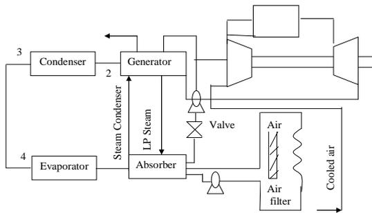
Figure 5: Schematic diagram of a gas turbine plant integrated with a vapour absorption refrigeration system
