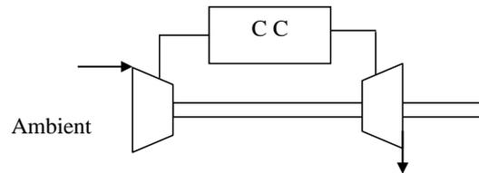
Figure 1: Schematic Diagram of the Standard Gas Turbine Cycle
