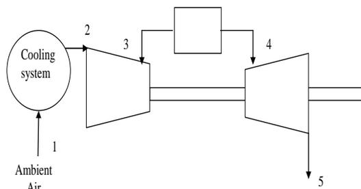
Figure 2: Schematic Diagram of a Gas turbine cycle with pre-cooling techniques
