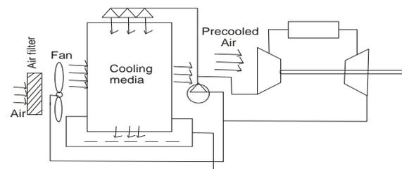
Figure 3: schematic diagram of an evaporative pre-cooling system integrated to a gas turbine plant
