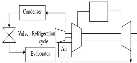
Figure 4: Schematic diagram of a gas turbine plant integrated with vapour compression system
