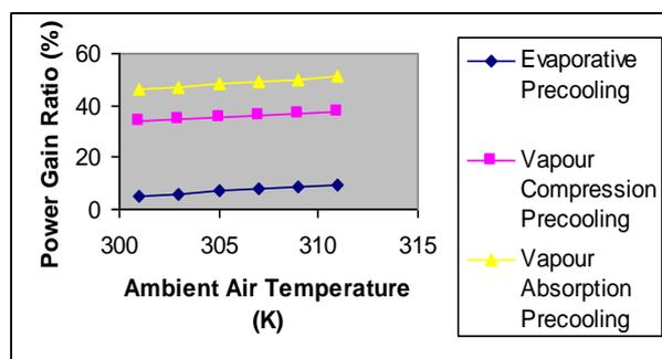
Figure 6: Variation of Power Gain Ratio (%) for the various pre-cooling techniques
