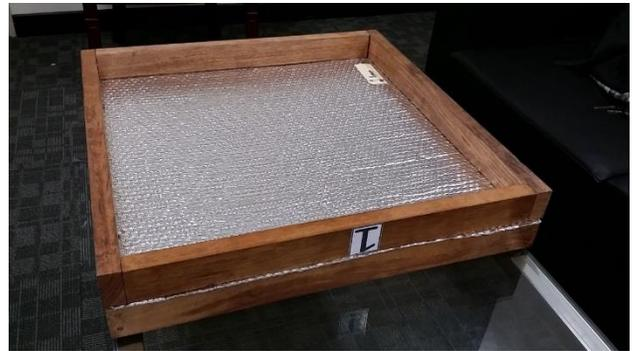
Fig 4 Timber frames are used to create top and bottom air gaps for bubble foil for heat flow meter measurement
