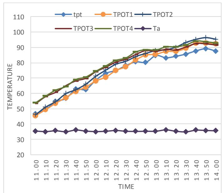
Fig. 5 Temperature profile of pots filled with daal and rice (cooking test)
