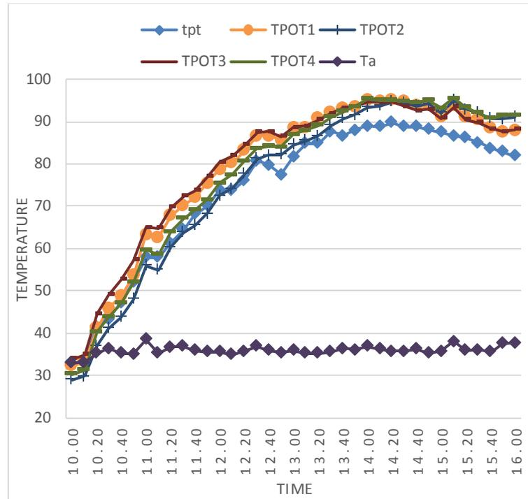
Fig. 4 Temperature profile of pots kept in the solar cooker (load test with water)
