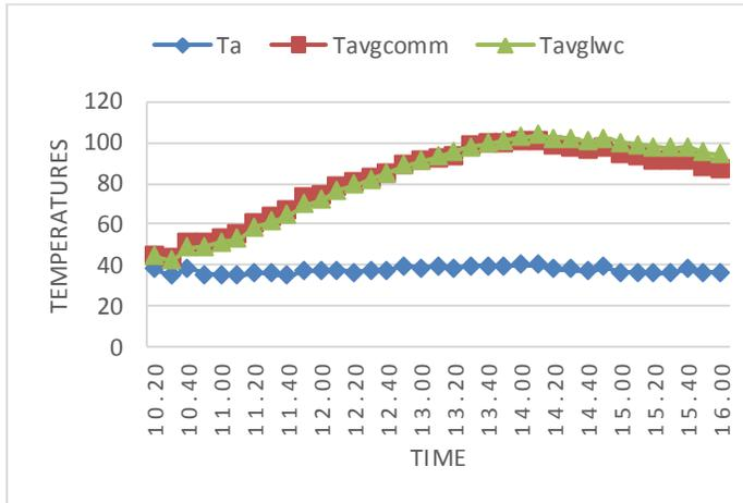
Fig. 2 Comparison of light weight cooker with commercial cooker. The experiments were conducted at Surat (21.15 N, 72.85 E)
