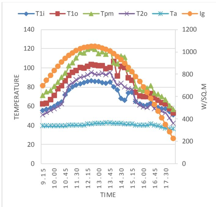
Fig. 3 Temperature profile of various components at no load test.
