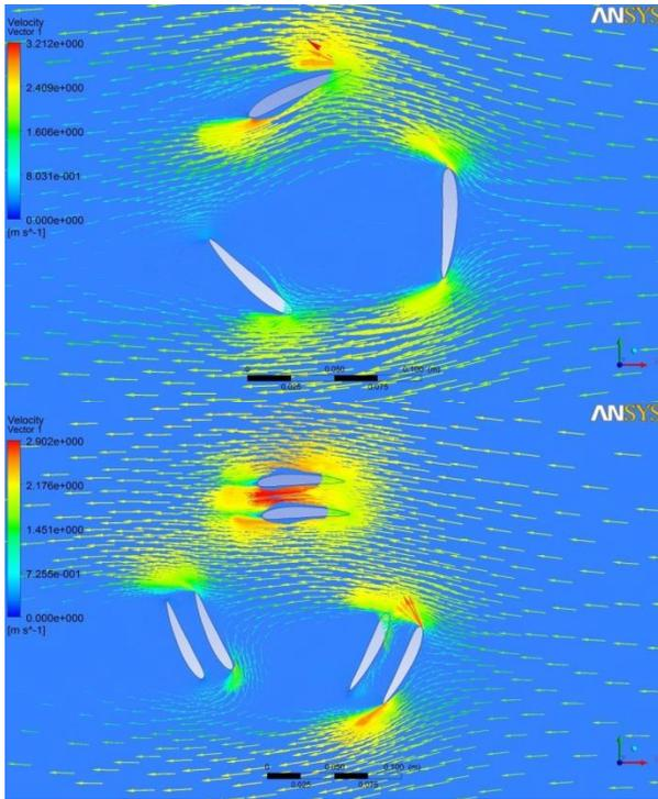
Fig. 6 Air velocity vectors with and without secondary blades
