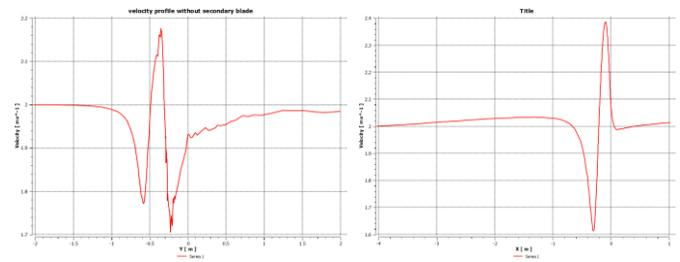
Fig. 5a Velocity profile without secondary blade.
