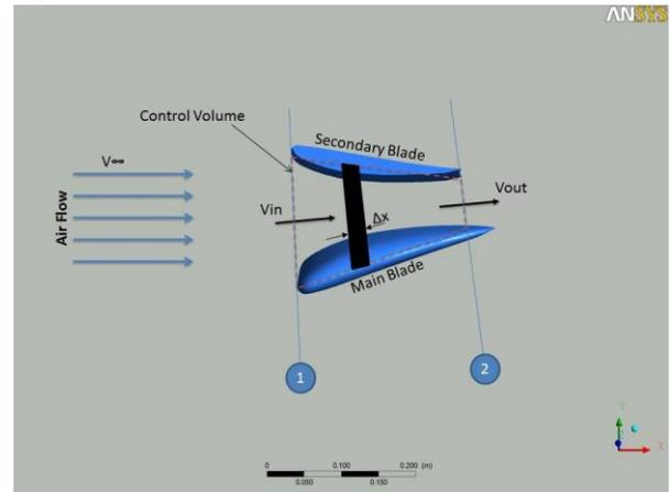
Fig. 3 Control volume of area between main and secondary blades
