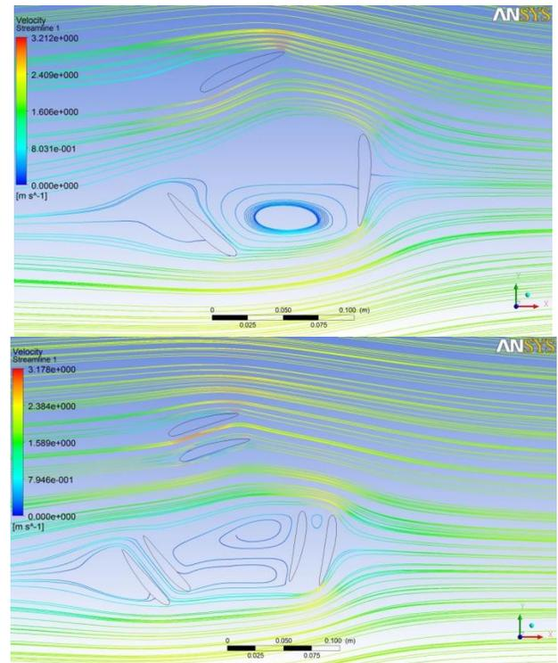
Fig. 4 Profile of velocity streamlines of original and developed vertical axis wind turbine
