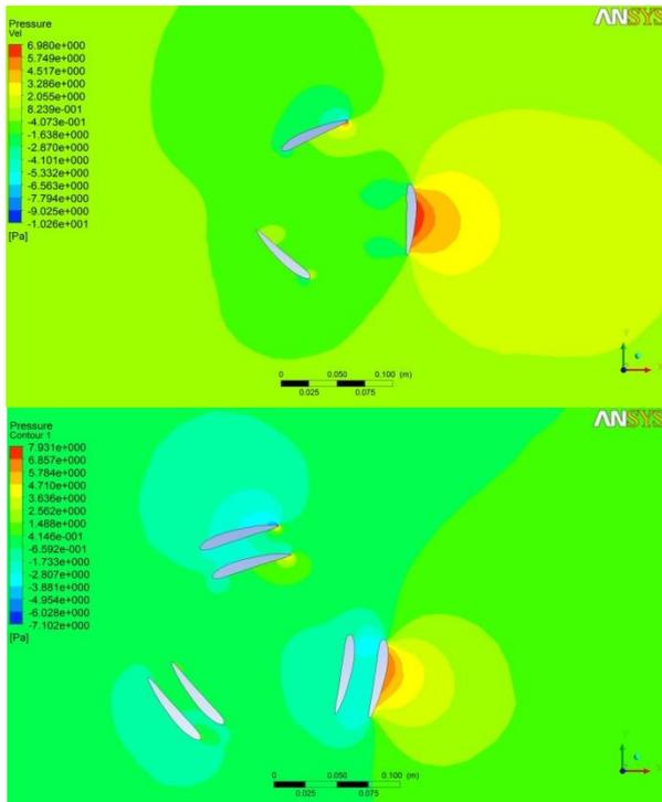
Fig. 7 Pressure distribution with and without secondary blade
