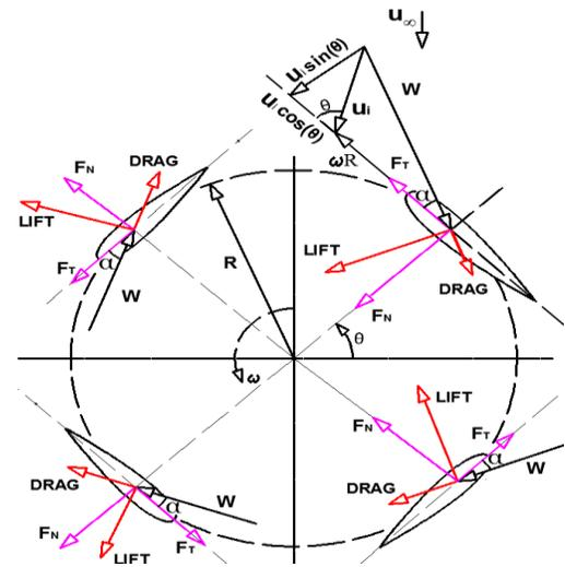
Fig. 2 Forces and velocity analysis in vertical axis wind turbine
