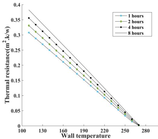
Fig. 4 The change of frost thermal resistance with different wall temperature.  $T_a = 20^\circ\text{C}$ ,  $\varphi = 50\%$ .
