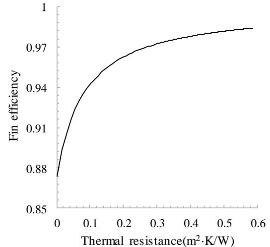
Fig. 5 The change of fin efficiency with thermal resistance. ( $T_a = -15^\circ\text{C}$ ,  $\varphi = 30\%$ ,  $T_w = 110\text{K}$ ,  $H = 80\text{mm}$ )
