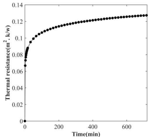
Fig. 1 The change of frost thermal resistance with time.
