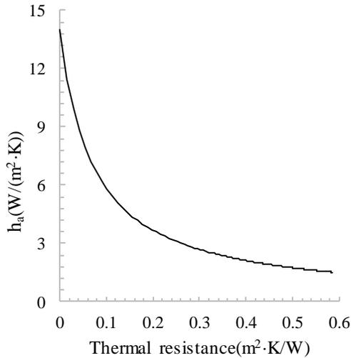
Fig. 6 The change of surface heat transfer coefficient of the fin with thermal resistance. ( $T_a = -15^\circ\text{C}$ ,  $\varphi = 30\%$ ,  $T_w = 110\text{K}$ ,  $H = 80\text{mm}$ )
