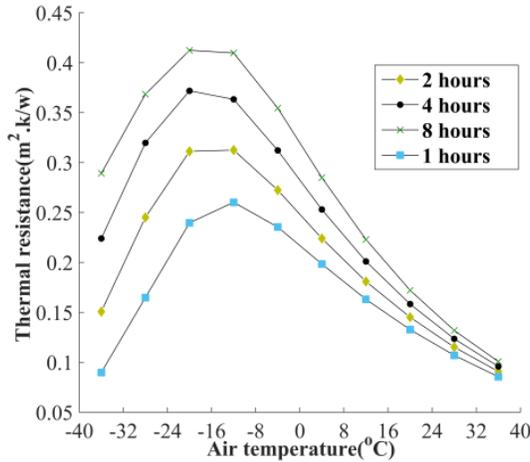
Fig. 2 The change of frost thermal resistance with different air temperature.  $\varphi = 50\%$ ,  $T_w = 200\text{K}$ .
