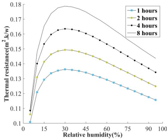
Fig. 3 The change of frost thermal resistance with different relative humidity.  $T_a = 20^\circ\text{C}$ ,  $T_w = 200\text{K}$ .
