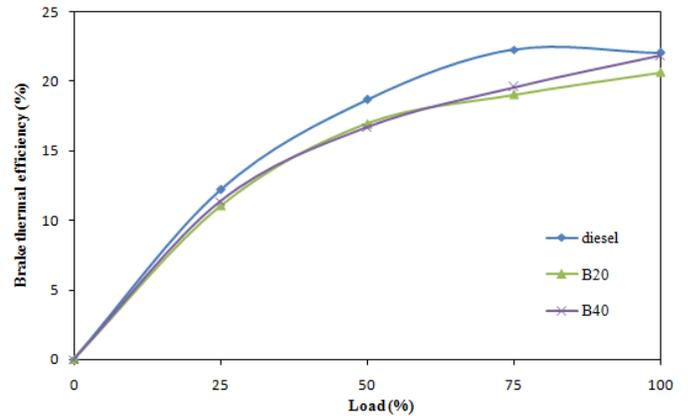
Fig.3 Comparison of brake thermal efficiency with load
