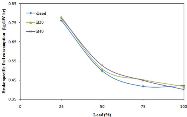
Fig. 2 Comparison of brake specific fuel consumption with load
