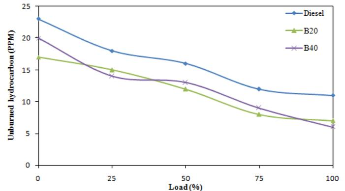
Fig.4 Comparison of Unburned hydrocarbon emissions with load
