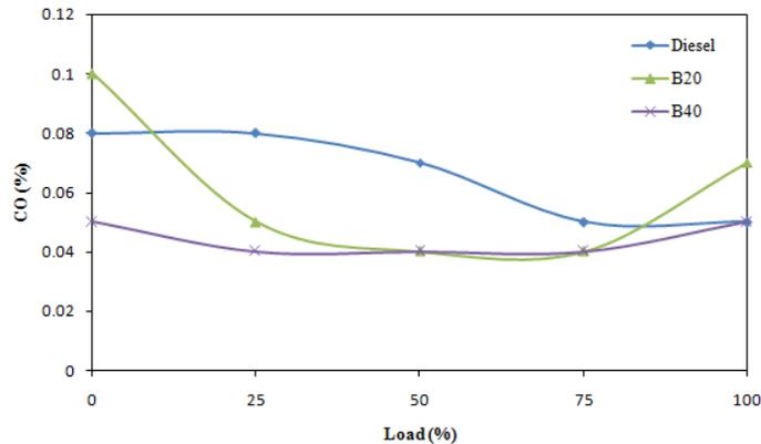
Fig.5 Comparison of Carbon monoxide emissions with load
