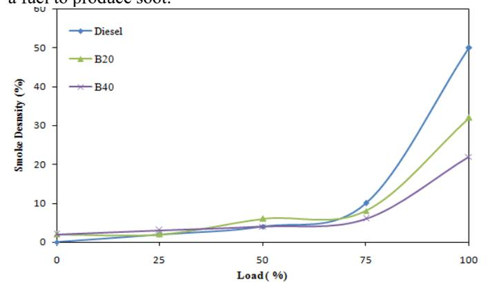
Fig.7 Comparison of Smoke emissions with load
