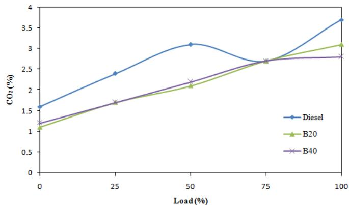
Fig.6 Comparison of Carbon dioxide emissions with load
