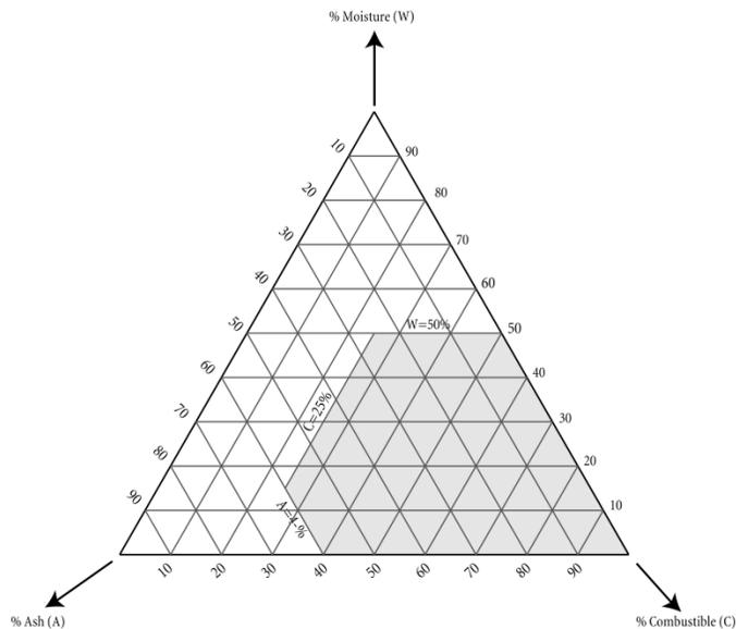
**Fig. 2 Tanner's diagram [7] of MSW incineration, the World Bank, Washington, D.C.**
