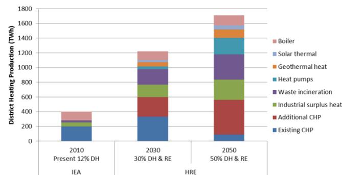
**Fig. 1 Waste incineration in district heating (DH) production for the EU27 energy system in 2010, 2030, and 2050, if DH and CHP were expanded to 30% in 2030 and 50% in 2050 [2].**
