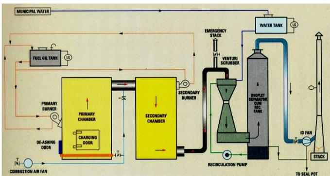
Fig. 3 Incinerator (semi-pyrolitic) setup [14].
