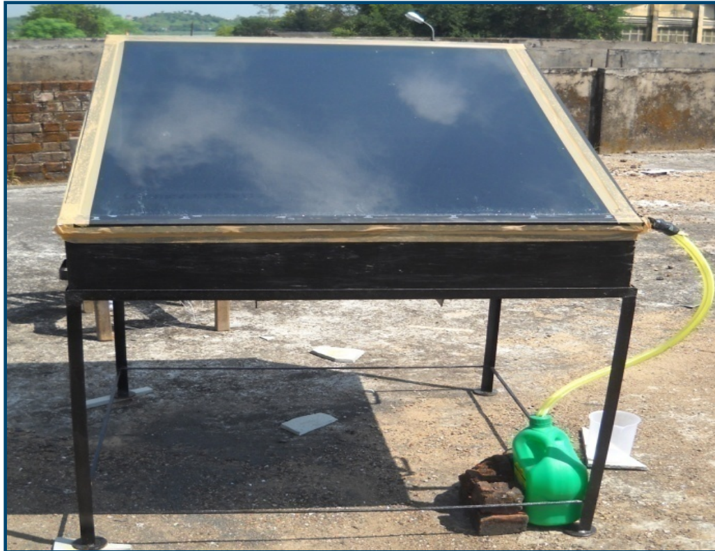
Figure : 3.1 Experimental Setup of Single Slope Solar Still
